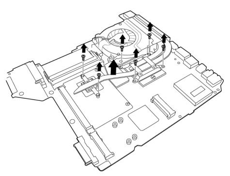
Figure 4-37 Removing screws securing heat sink
